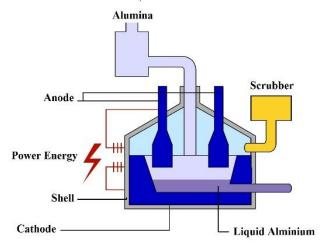
Fig 2- View of the cross-section of an electrolysis
